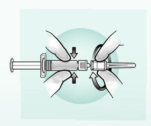
Hold the syringe barrel in one hand and **unscrew the syringe tip cap** by twisting it **counterclockwise. Attach a needle** by **twisting clockwise** until the needle fits securely on the syringe.
